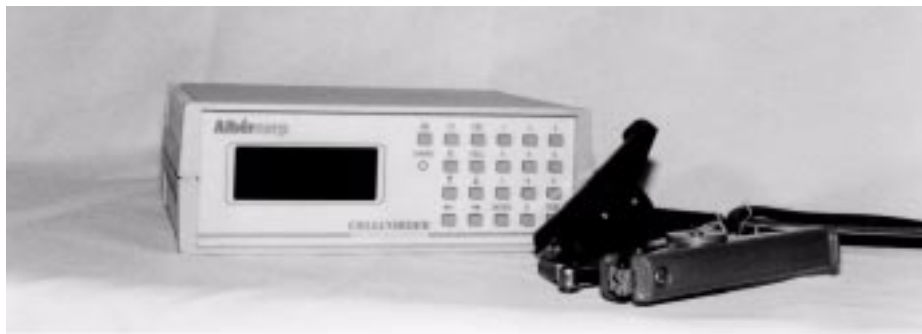
Figure 7.4. Internal Resistance Tester.
