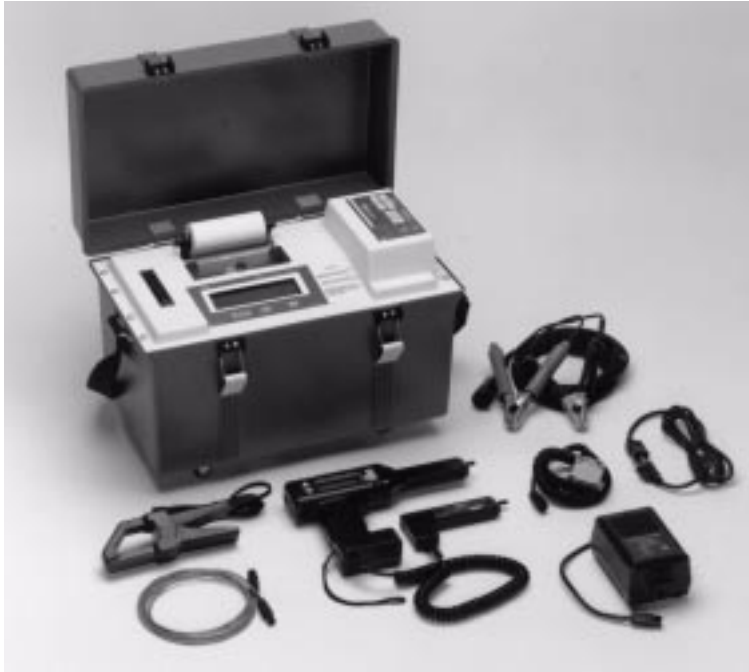
Figure 7.3. Internal Impedance Tester.
