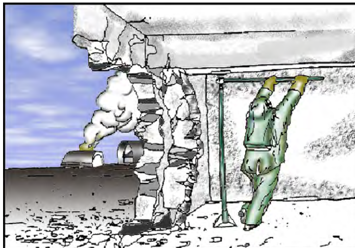
Figure 3.13. Shoring Jack Installation.
