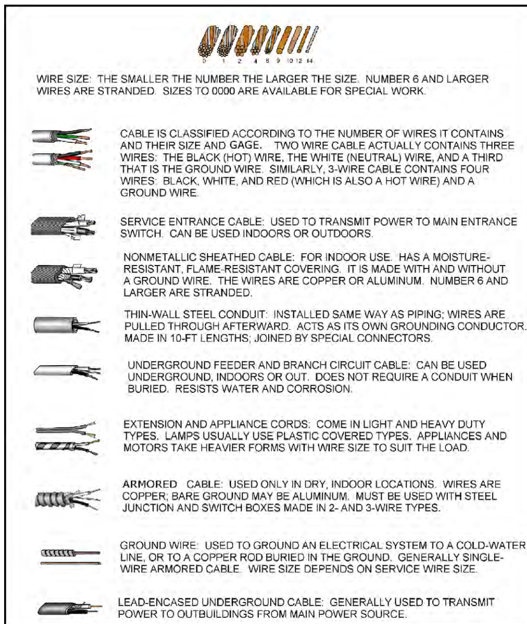
Figure 5.20. Wire Sizes, Types, and Uses.
