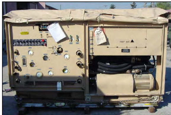
Figure 4.12. 600-GPH Reverse Osmosis Water Purification Unit (ROWPU).
