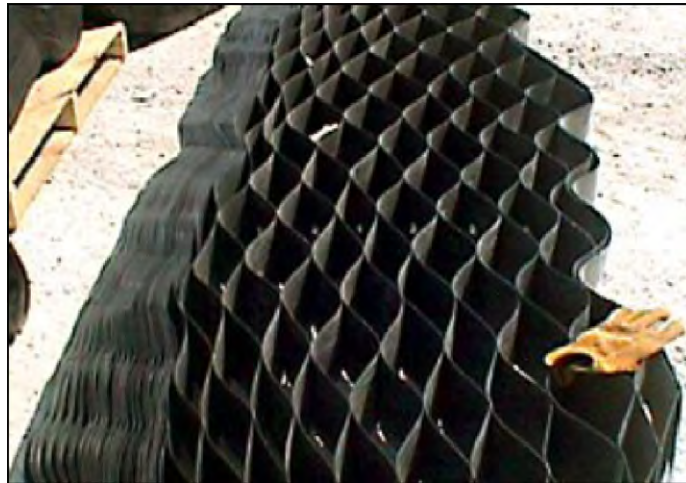
Figure 2.2. Typical Sand-Grid Material in Shipping Configuration.
