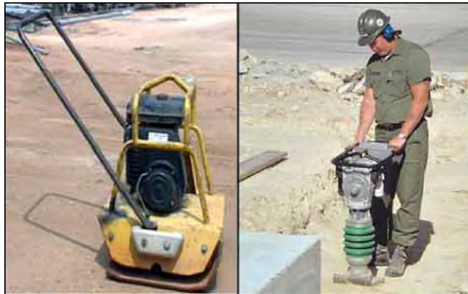
Figure 7.4. Portable Vibratory Compactors.
