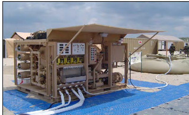
Figure 4.13. 1500-GPH Reverse Osmosis Water Purification Unit (ROWPU).
