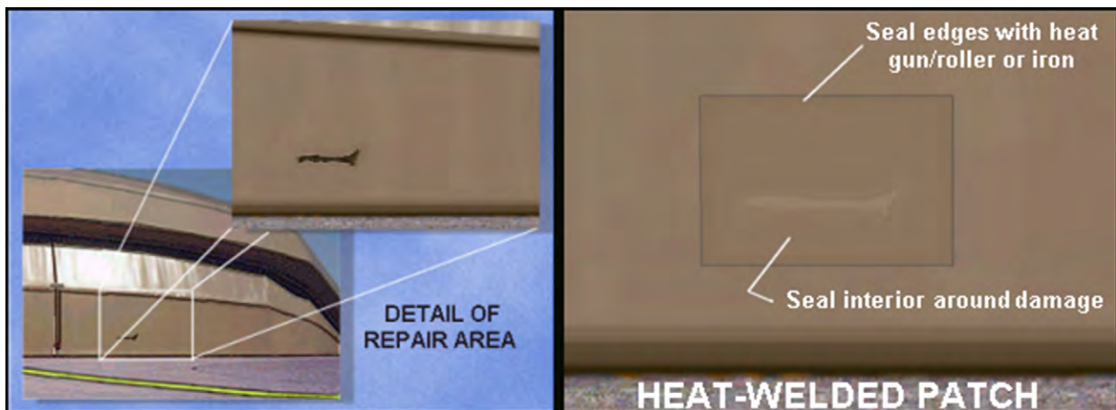
Figure 3.35. Typical Heat/Solvent -Welded Patch Repair.
