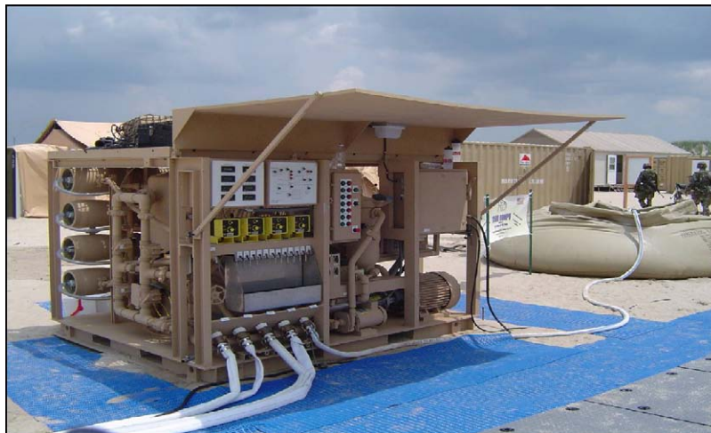
Figure 6.7. 1500-GPH Reverse Osmosis Water Purification Unit (ROWPU).
