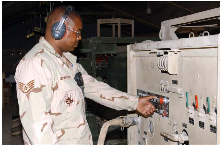
Figure 6.6. 600-GPH Reverse Osmosis Water Purification Unit (ROWPU).
