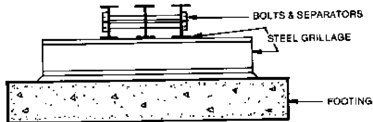
Figure 2-5. STEEL GRILLAGE FOUNDATION.
