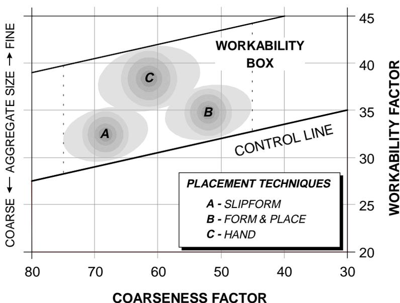
Figure 3.3 Workability Box Within Aggregate Proportioning Guide
