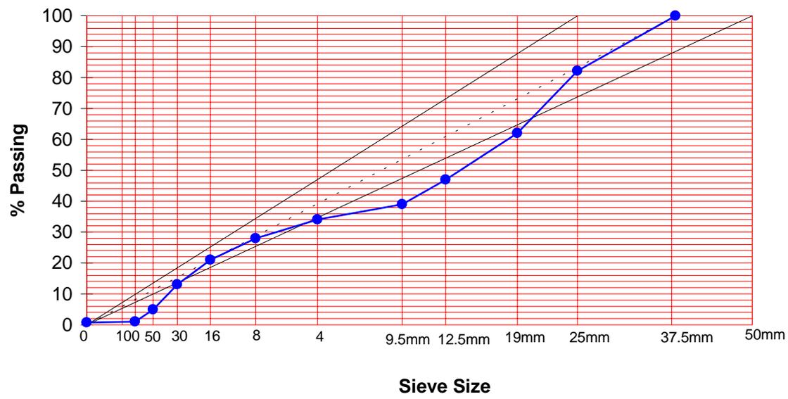
Figure 3.10 Example C Plotted on 0.45 Power Chart
