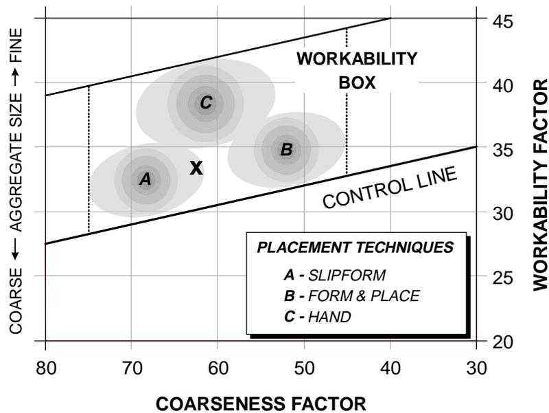
Figure 6.7 Aggregate Proportioning Guide for Combined Aggregate
