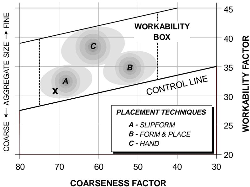
Figure 6.3 Aggregate Proportioning Guide for Combined Aggregate
