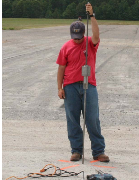
Figure 3. Using a DCP to Determine Subgrade Soil Strength
