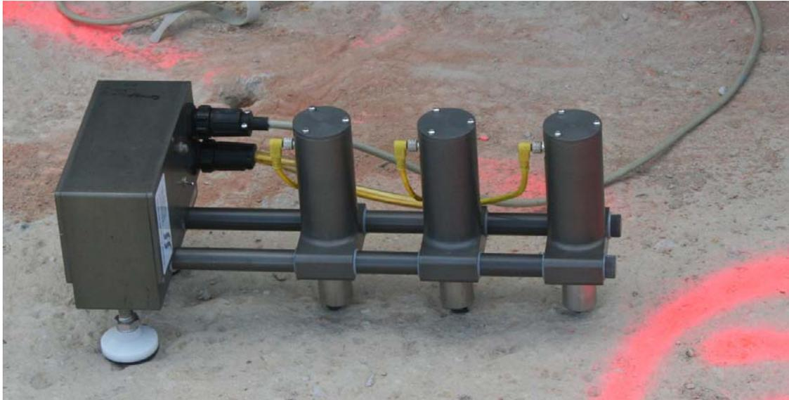
**Figure 1. Portable Seismic Property Analyzer (PSPA)**
