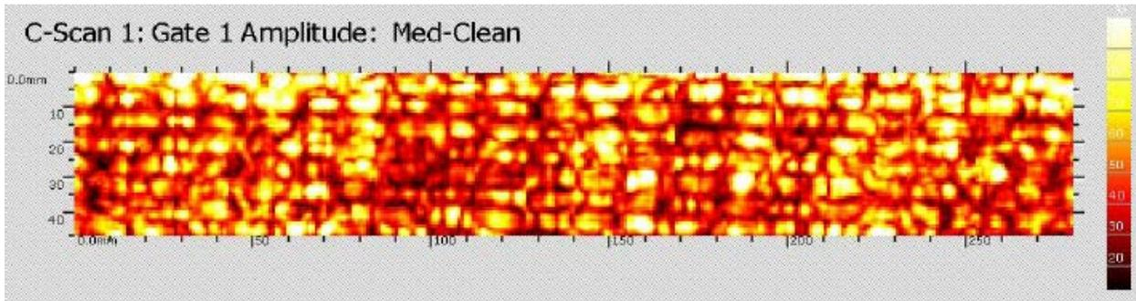
**Figure 11. Example of C-Scan Plot Showing Results for Undamaged FFM**
