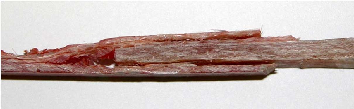
Figure 15. Cross-Section of Failed Secondary Bond Test Specimen
