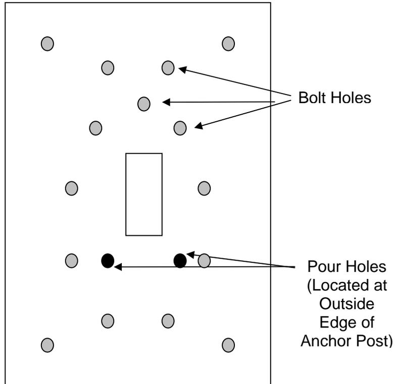
**Figure 13. Top View of Anchor Test Plate with Bolt and Pour Holes
