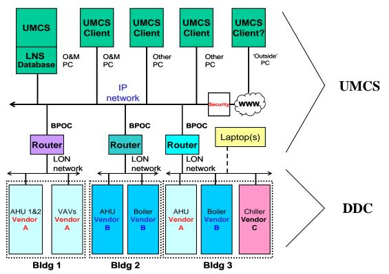
Figure 1. Basewide LONWORKS<sup>®</sup> BAS—including a UMCS and multiple-vendor DDC systems.
