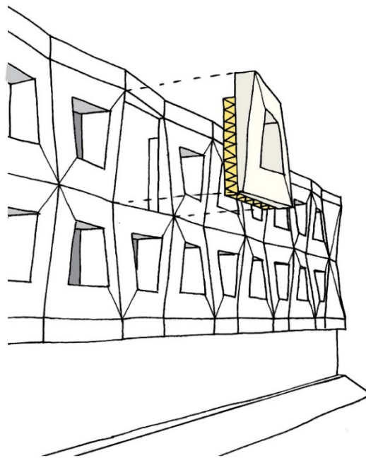
Figure H-12. Detail of panel module.
