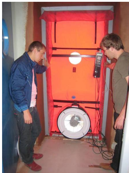
Figure C-13. Building-time blower-door test, the value n_{50} = 0,47 1/h was reached.
