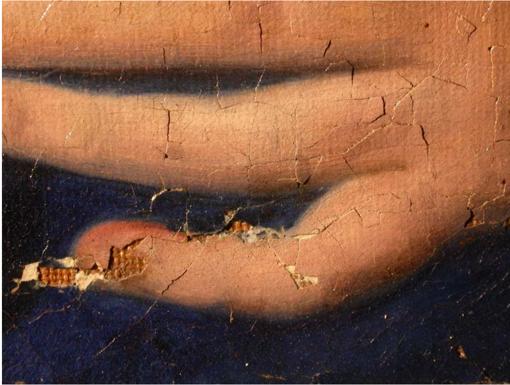
Figure 46 shows a detail of a 19 th century Italian painting. It is clear that total separation of the paint and ground layers from the canvas has occurred. The moisture was sufficient to cause the adhesive bond of the animal glue size layer to completely fail. (Photo by Matteo Rossi Doria)
