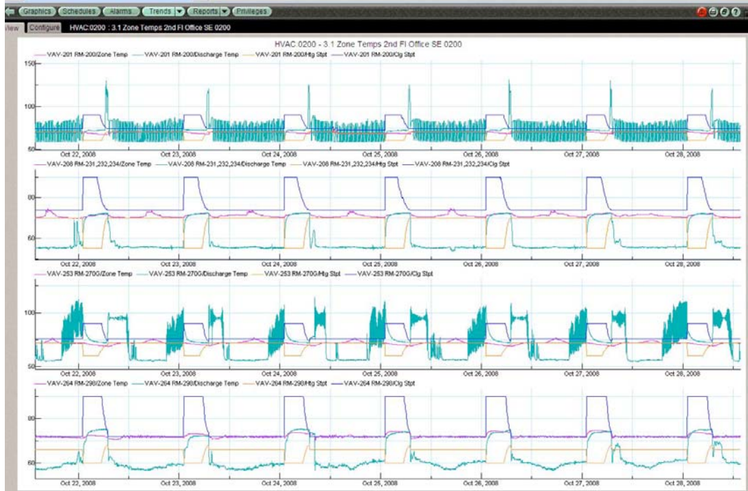
Figure 3: Diagnostic trends of VAV zone temperatures
